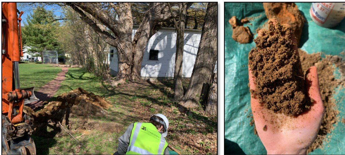
Figure 4. Soils investigation (left) and sample of soil at a depth of 10-in (right).
