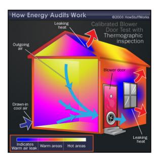
Thermographic inspections use infrared cameras to identify where heat is escaping from your home. The heat shows up on the camera as white, yellow and red. Sometimes this test is done together with the calibrated blowers test.
