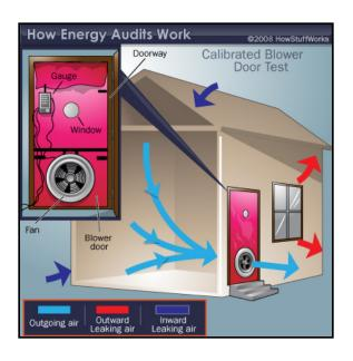
The test attaches a fan to the outside door. The fan pulls air out of the house to lower the inside air pressure. Air from the outside flows in through any openings. While the air is being pulled out, the auditor can see where the leaks are occurring.
