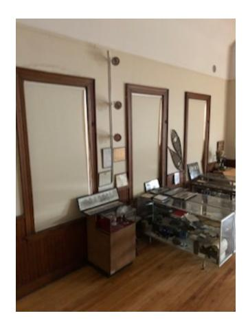
Due to Stack Effect the windows are a large area of concern with warm air being pushed through cracks and gaps, the installation of interior storm panels will reduce the losses, these interior storm panels can be removed to allow for cleaning but offer a needed air barrier, unlike the second floor shades, this type of window treatment can be ordered with UV film to protect from damaging sun light.
