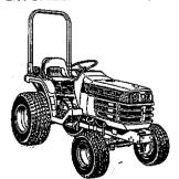
4WD, 16 Horsepower Diesel Hydrostatic Drive Front Bucket Loader (LA272) 60" belly Mower with Bagging System 4' Scraper Blade, Drawbar Live Hydraulics, 2 speed PTO, 3 Point Hitch
